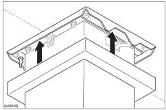
■ Finally, being careful not to scratch the chimney, push the cover plate upwards until the spring fixing clips click into place. If installed correctly, the cover should be secure and flush against the ceiling.
